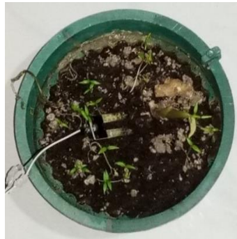
Gambar 17 Pengujian Soil Moisture Sensor
